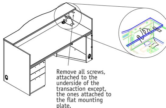
Remove all screws, attached to the underside of the transaction except, the ones attached to the flat mounting plate.
